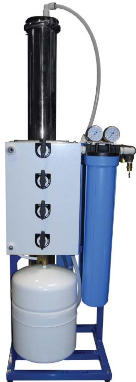
The EE-UF system purifies drinking water without electricity using a minimum of 35 psi feed pressure. EE-UF-5000 system shown above.
